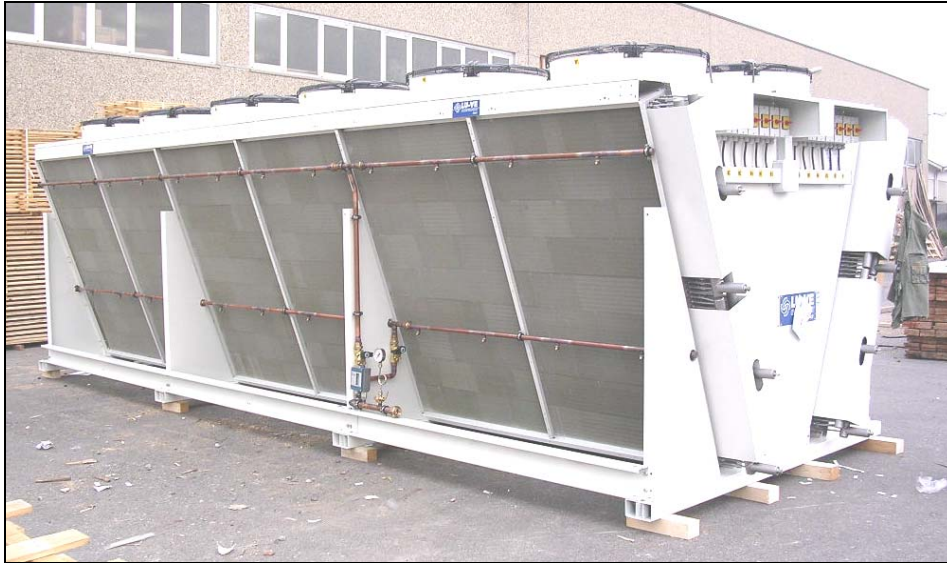
Fig.4: A large CO 2 gas cooler ready for shipping at LU-VE workshop.
